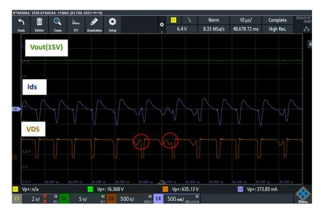
This is not double switching. This means that the TRF is now operating in discontinuous mode.
