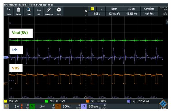
b) Why does Ids current waveform look abnormal (even when SMPS is working fine) – Current seems to rise during FET off time. [ Note – Direction and placement of the probe is correct]
