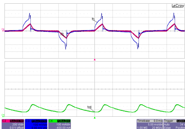
Figure 86 – 240 VAC / 50 Hz, (Germany) Busch 6513 U102 Dimmer at minimum TRIAC Conduction. Load: 36 V LED String. Ch2: V_{IN} , 200 V / div. Ch3: I_{IN} , 100 mA / div. Ch4: I_{OUT} , 100 mA / div. Time Scale: 5 ms / div.
