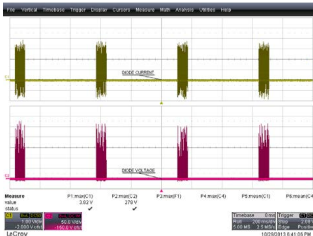
Figure 54 – 265 VAC, 50 Hz. Upper: I_{D7} , 1 A / div. Lower: V_{D7} , 50 V / div., 200 ms / div.
