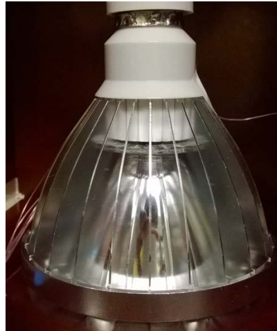
Figure 23 – Actual LED Enclosure Used in Thermal Verification.
