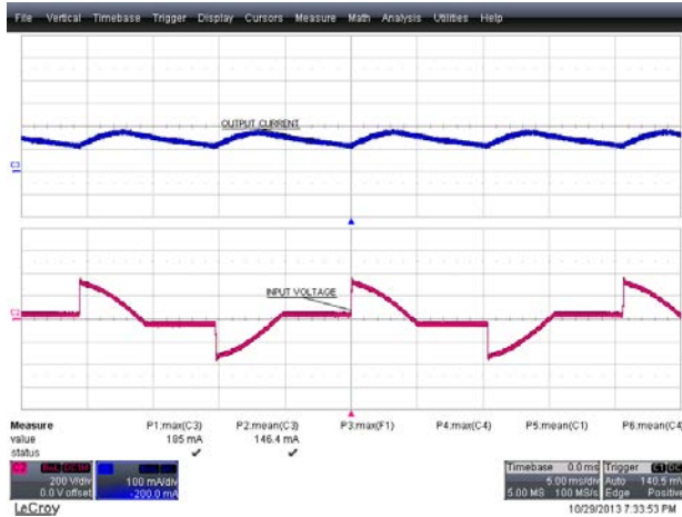
Figure 64 – 90° Conduction Angle. Upper: I_{OUT} , 100 mA / div. Lower: V_{IN} , 200 V, 5 ms / div.
