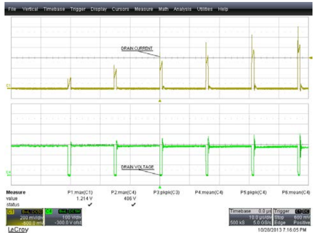
Figure 42 – 265 VAC, 50 Hz Start-up. Upper: I_{DRAIN} , 200 mA / div. Lower: V_{DRAIN} , 100 V, 10 μs / div.
