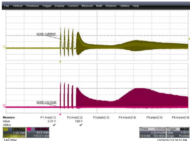
Figure 51 – 195 VAC, 50 Hz. Upper: I_{D7} , 1 A / div. Lower: V_{D7} , 50 V, 2 ms / div.
