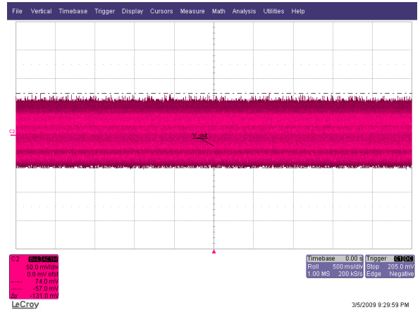
Figure 71 – Ripple, 265 VAC, Full Load. 500 ms / div, 50 mV / div.
