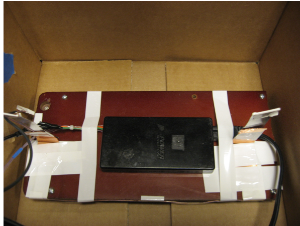
Figure 35 – Power Supply Adapter Inside Carton Box and on Top of Bakelite Board for Burn-In Test.
