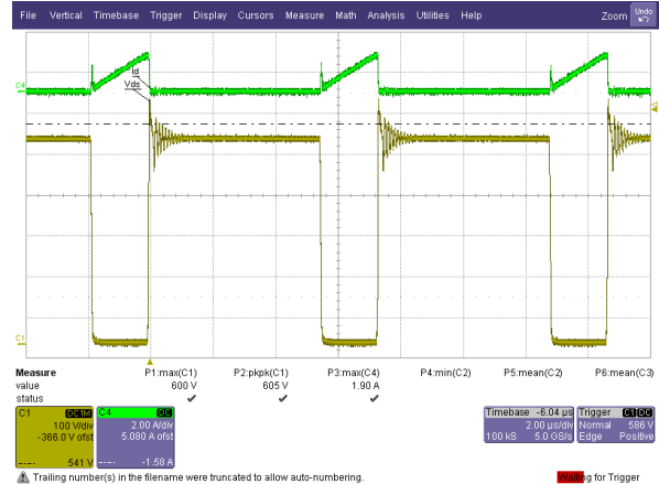
Figure 45 – 265 VAC, Overload Condition. With OCP Protection. Upper: I_{DRAIN} , 2 A / div. Lower: V_{DRAIN} , 200 V / div.
