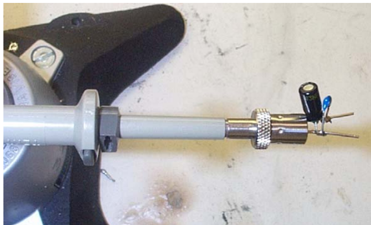
Figure 19 – Oscilloscope Probe with Probe Master 5125BA BNC Adapter. (Modified with wires for probe ground for ripple measurement, and two parallel decoupling capacitors added).
