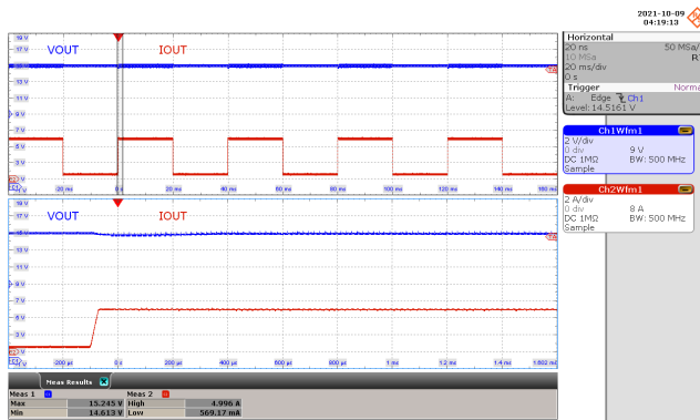
Figure 108 – Transient Response. 90 VAC, 15.0 V, 0.5 to 5 A Load. V_{OUT} = 15.24 \text{ V Max.}, 14.61 \text{ V Min.} CH1: V_{OUT}, 2 \text{ V / div.} CH2: I_{OUT}, 2 \text{ A / div.} Time: 20 ms / div. (200 \mu\text{s} / div. Zoom).
