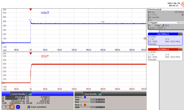
Figure 70 – Output Voltage and Current. 90 VAC, 5.0 V, 5 A (CR Mode, 880 mΩ at the End of 100 mΩ Cable). V_{OUT} = 4.4625 V Steady-State. CH1: V_{OUT} , 1 V / div. CH2: I_{LOAD} , 1 A / div. Time: 40 ms / div.
