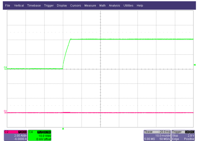
Figure 16 – Output Voltage Start-up – No-Load 265 VAC. C4 – Output Voltage – 5 V / div. C2 – Output Current – 1 A / div. 10 ms / div.
