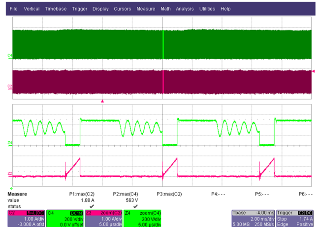
Figure 20 – Drain Voltage and Current Waveforms. 265 VAC, 100% Load, (563 V_{MAX} ). C4/Z4: V_{DRAIN} , 200 V / div., 2 ms / div. C2/Z2: I_{DRAIN} , 1 A / div.
