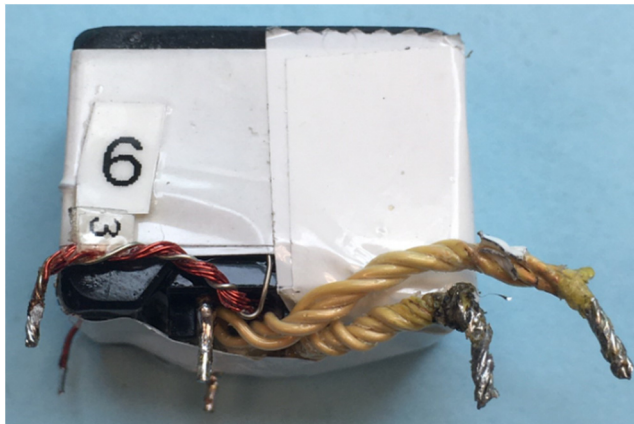
Cut transformer flying leads to required length and tin the flying leads
