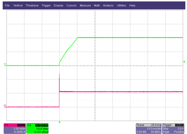
Figure 14 – Output Voltage Start-up – 100% Load 265 VAC. C4 – Output Voltage – 5 V / div. C2 – Output Current – 1 A / div. 10 ms / div.
