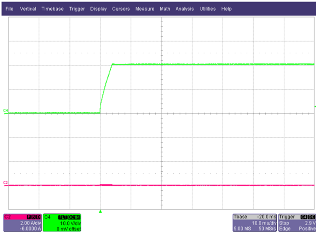
Figure 15 – Output Voltage Start-up – No-Load 90 VAC. C4 – Output Voltage – 5 V / div. C2 – Output Current – 1 A / div. 10 ms / div.
