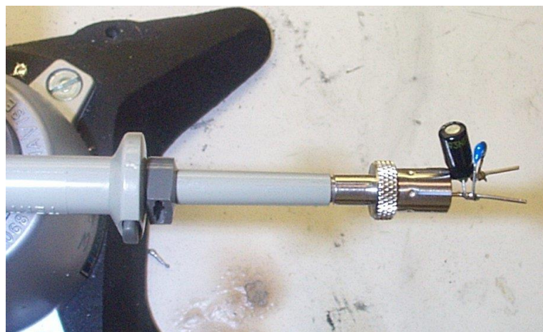
Figure 81 – Oscilloscope Probe with Probe Master ( www.probemaster.com ) 4987A BNC Adapter. (Modified with wires for ripple measurement, and two parallel decoupling capacitors added.)
