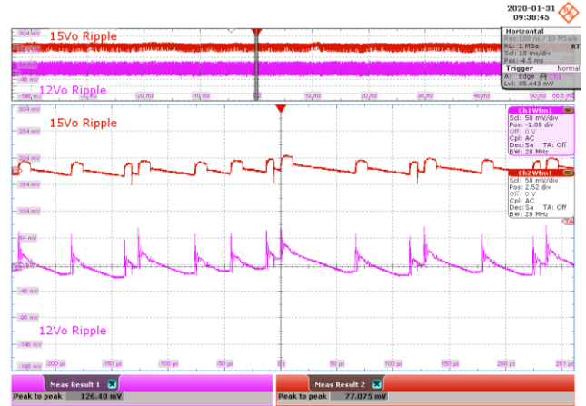
Figure 91 – 115 VAC 60 Hz. CH1: V_{12V\_OUT} , 50 V / div., 10 ms / div. CH2: V_{15V\_OUT} , 50 V / div., 10 ms / div. Zoom: 50 \mu s / div. 12 V Output Ripple = 126.48 mV. 15 V Output Ripple = 77.075 mV.
