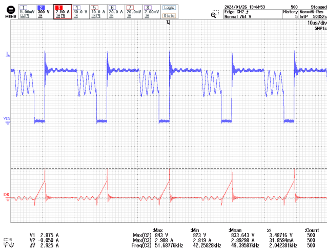
Figure 59 – INN3949CQ Drain Voltage and Current. Vin = 190 V DC , 5 A Load. CH2: V DS,INNO , 300 V / div. CH3: I DS,INNO , 2.5 A / div. Time: 10 µs / div.
