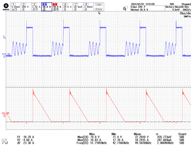
Figure 62 – SR FET Drain Voltage and Current. Vin = 190 V DC , 5 A Load. CH2: V DS,INNO , 30 V / div. CH3: I DS,INNO , 10 A / div. Time: 10 μs / div.
