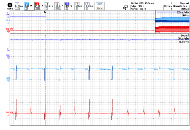
Figure 40 – INN3949CQ Drain Voltage and Current. 450 V DC , 2.8 Ω Load. CH6: V IN , 300 V / div. CH2: V OUT , 500 V / div. CH3: I OUT , 2 A / div. Time: 20 ms / div.
