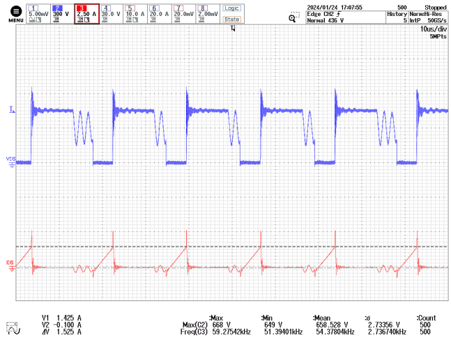
Figure 54 – INN3949CQ Drain Voltage and Current. Vin = 300 V DC , 5 A Load. CH2: V DS,INNO , 300 V / div. CH3: I DS,INNO , 2.5 A / div. Time: 10 µs / div.
