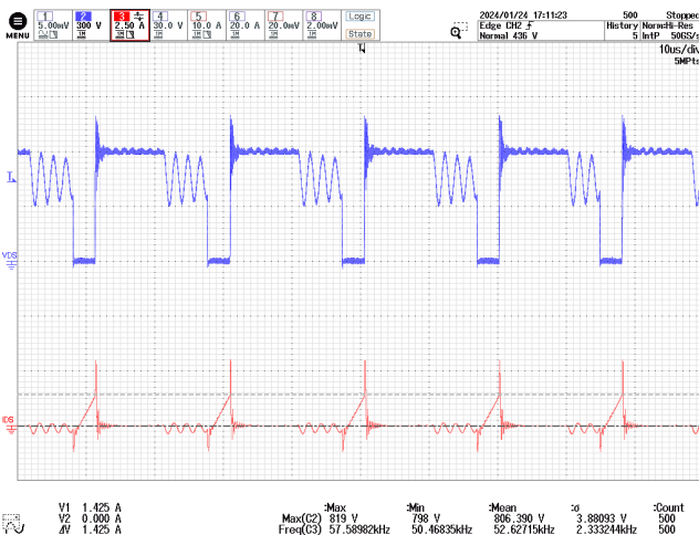
Figure 53 – INN3949CQ Drain Voltage and Current. Vin = 190 V DC , 5 A Load. CH2: V DS,INNO , 300 V / div. CH3: I DS,INNO , 2.5 A / div. Time: 10 µs / div.
