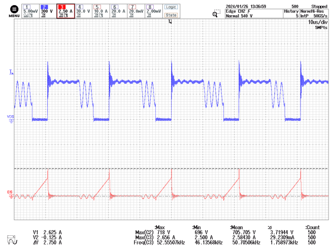
Figure 60 – INN3949CQ Drain Voltage and Current. Vin = 300 V DC , 5 A Load. CH2: V DS,INNO , 300 V / div. CH3: I DS,INNO , 2.5 A / div. Time: 10 µs / div.
